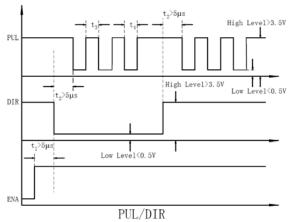
Figure 10: Sequence chart of control signals
